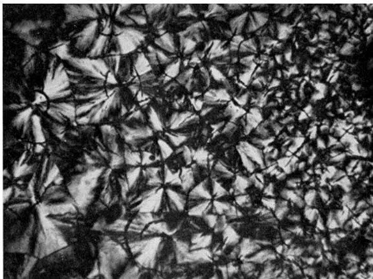
Fig. 2. Photomicrograph of poly-3-MB film after melting and slow cooling.
